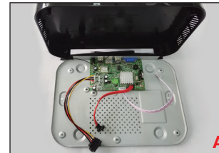
Unplug your NVR from power, unscrew and remove the top cover.
