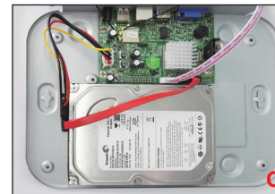
Place the HDD into the NVR. Any cable should cross up over the HDD.
