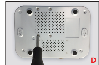
Holding the hard drive and the NVR, gently turn it over and line up the holes on the hard drive with the holes on the NVR. Using a Phillips screwdriver, screw the provided screws into the holes. Assemble the cover.
